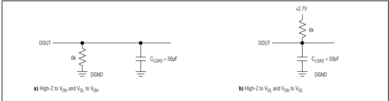
Figure 1. Load Circuits for DOUT Enable Time
