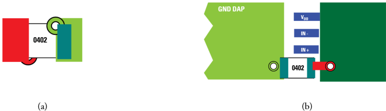
Figure 30. Typical Decoupling Capacitor Layouts
