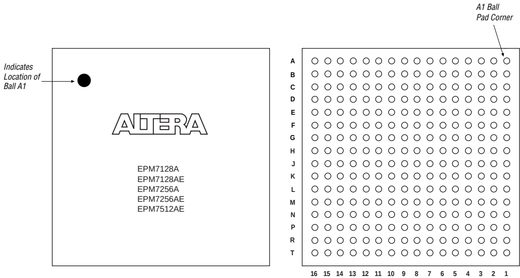
Figure 23. 256-Pin FineLine BGA Package Pin-Out Diagram
