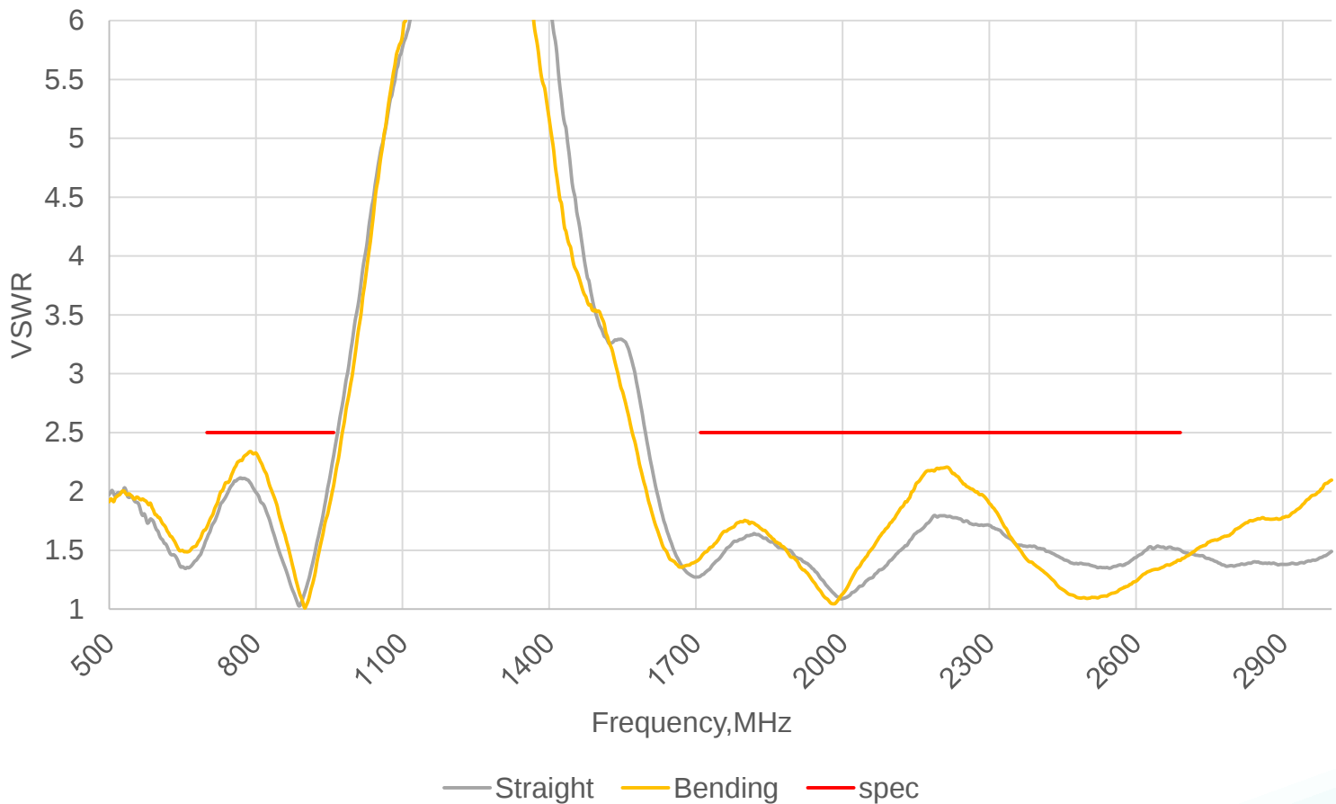
VSWR vs Frequency IceBladeLT measured in PSU
