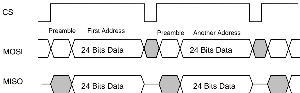
Figure 3. SPI Transfer Protocol Multiple Read/Write Access
