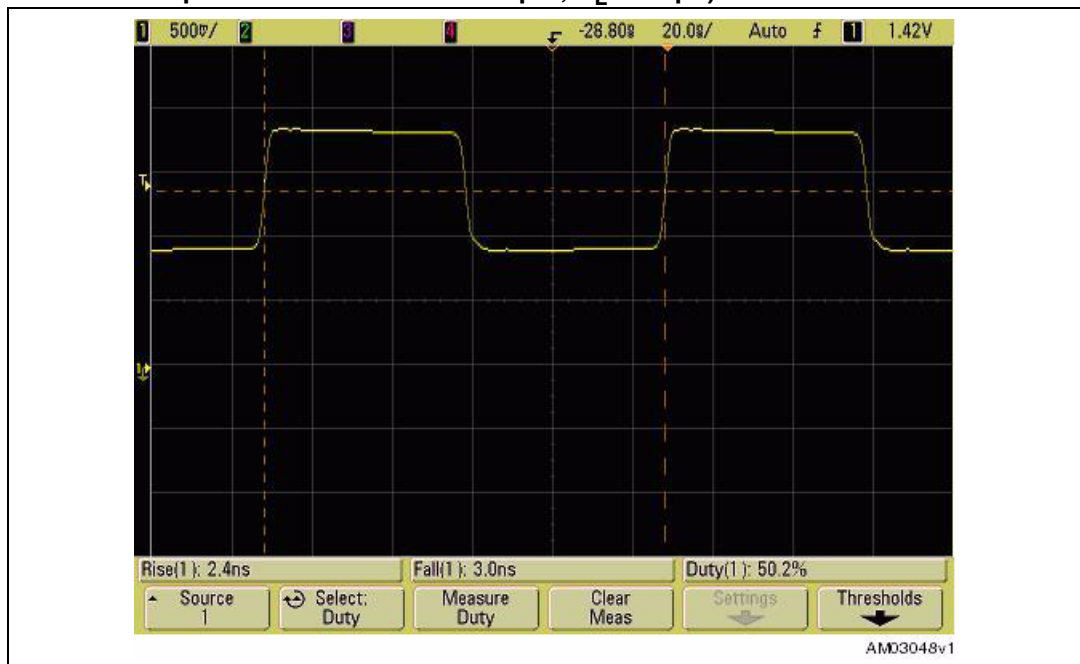
Figure 20. Rise and fall time for square wave output (STCD1040, 2.8 V, 10 MHz square wave master clock input, C_L = 20 pF)
