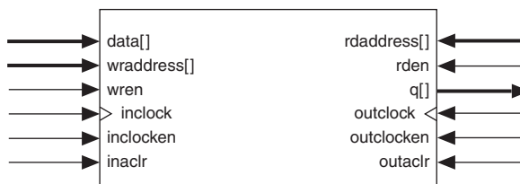
Figure 2–13. Simple Dual-Port and Single-Port Memory Configurations
