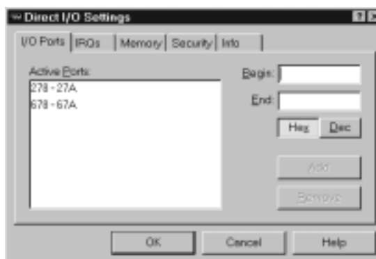
Figure 6. Correct I/O Addresses for LPT2 Access
