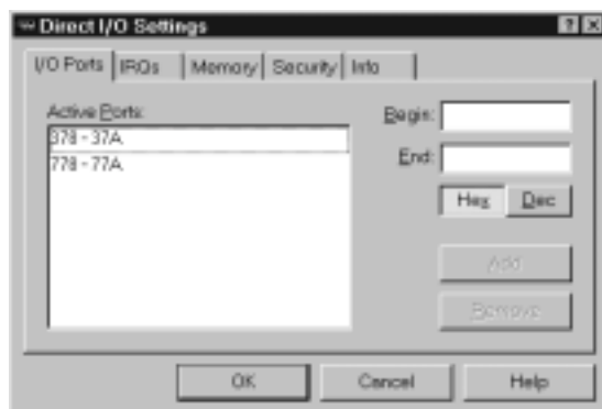
Figure 5. Correct I/O Addresses for LPT1 Access
