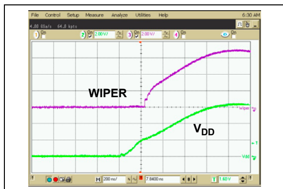
FIGURE 2-15: 2.1 k \Omega – Power-Up Wiper Response Time.
