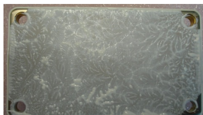
Picture 3: Grease on the module after disassembling.
