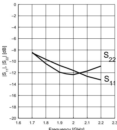
**Typical measurement results MID Gain Mode;  $T_A = 25^\circ\text{C}$**
