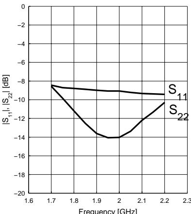
**Typical measurement results LOW Gain Mode;  $T_A = 25^\circ\text{C}$**
