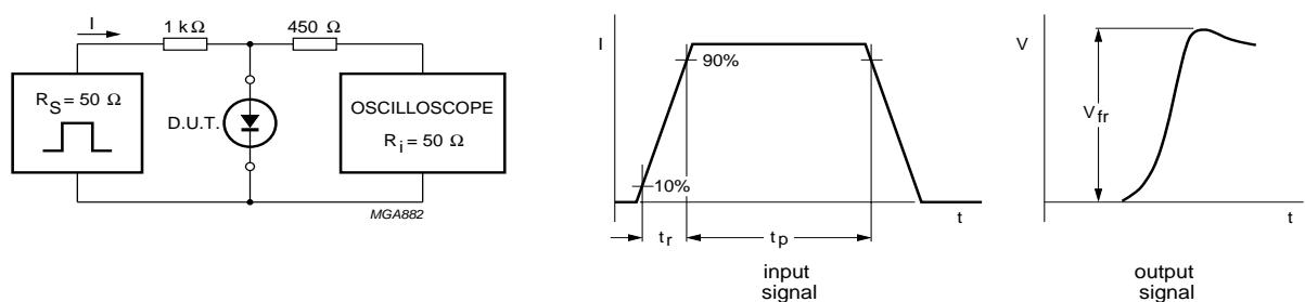
Fig.7 Forward recovery voltage test circuit and waveforms.
