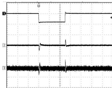
Channel 1: V_{IN} (500mV/div) Channel 2: V_{OUT} (500mV/div) Channel 3: I_{LED} (500μA/div) V_{IN} From 3.6 V To 3.2 V Time Base (400μs/div) L = 22\text{ }\mu\text{H} I_{LED} = 19\text{ mA}
