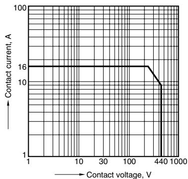
2. Max. switching power (DC resistive load)
