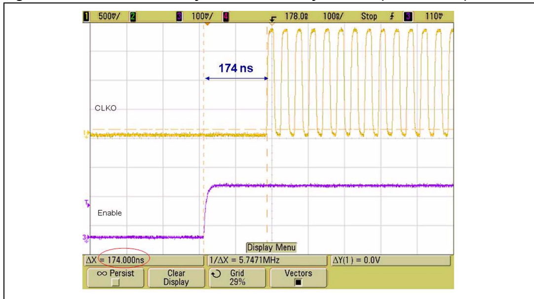
Figure 19. STCD2400 recovery time from off to on (VTCXO first in standby)
