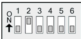
Figure B-17 RS-485 (4-wire) and RS-422 DIP Switch Settings
