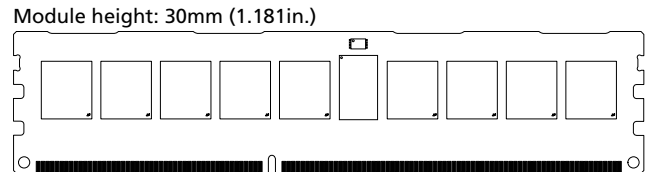
Figure 2: 240-Pin RDIMM (MO-269 R/C B1)
