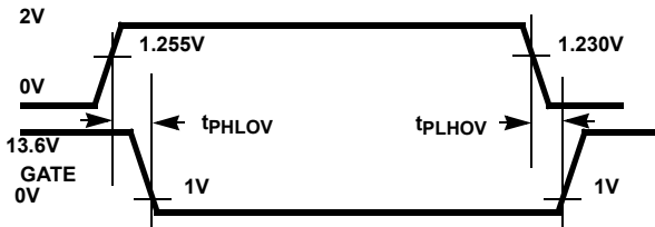
FIGURE 3A. OV TO GATE TIMING
