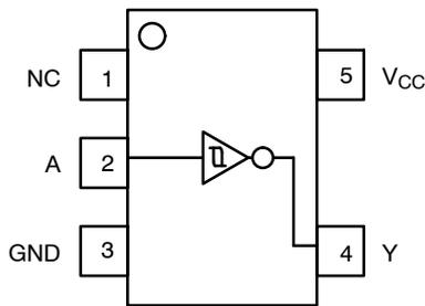
Figure 1. Pinout
