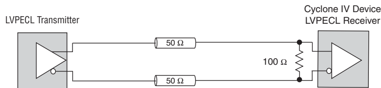
Figure 6-19. LVPECL DC-Coupled Termination (1)
