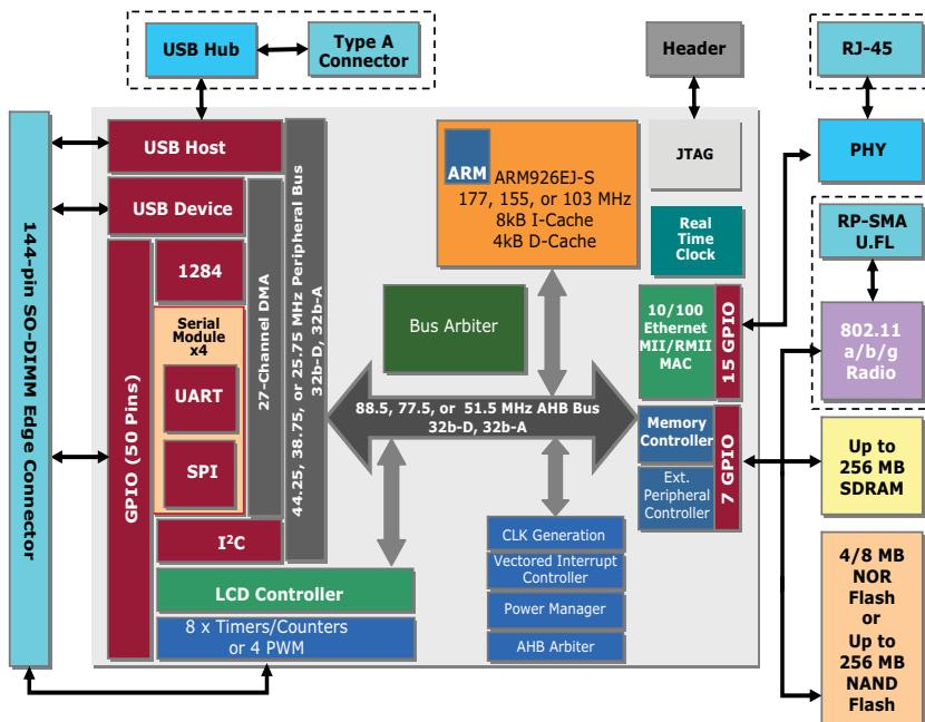
Highly integrated, compact ARM® core module family based on the powerful Digi NS9360 processor. Combines main processing functionality and integrated peripherals with on-board secure wireless/wired network connectivity.
