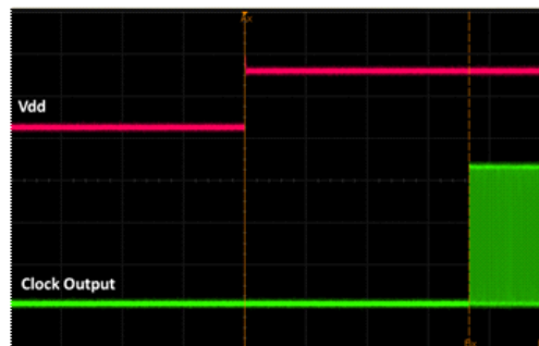
Figure 17. Startup Waveform vs. Vdd
