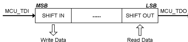
Figure 17-3 JTAG Port Shift Register
