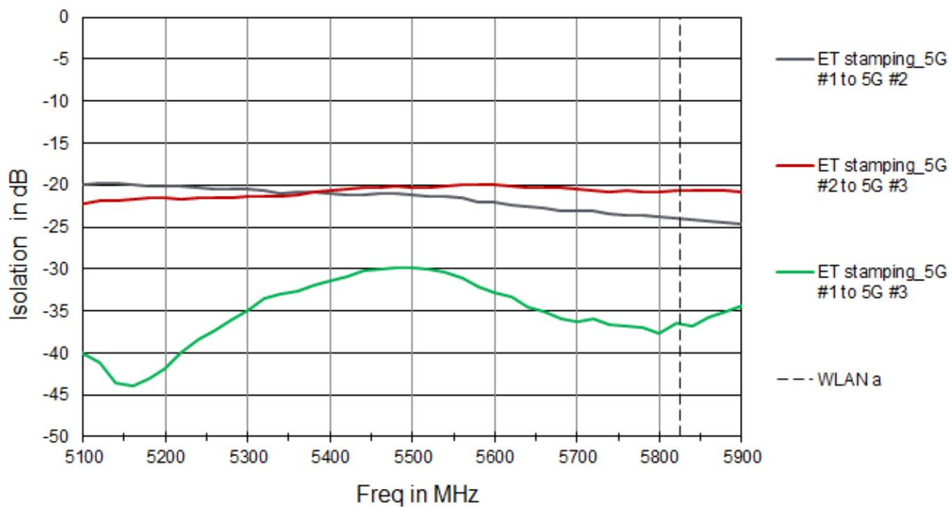
Isolation between each of the three antennas is below -20dB.
