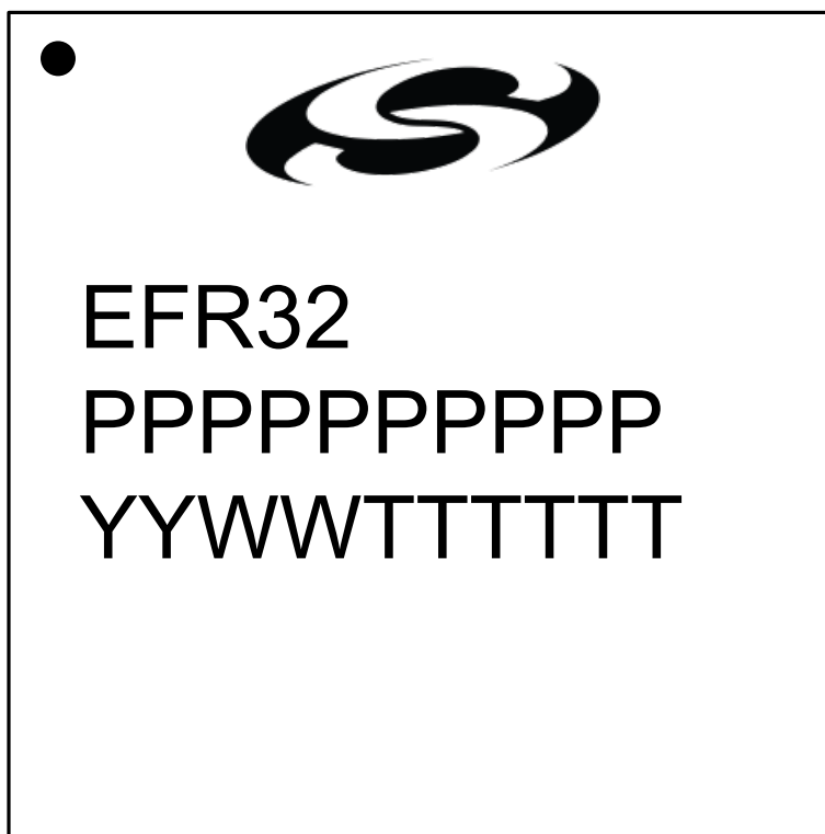
Figure 7.3. BGA125 Package Marking
