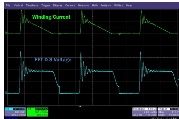
FIGURE 16. QUASI-RESONANT NEAR-ZVS SWITCHING
