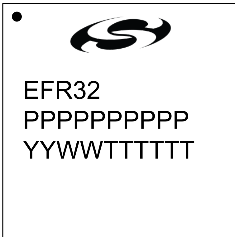
Figure 7.3. BGA125 Package Marking
