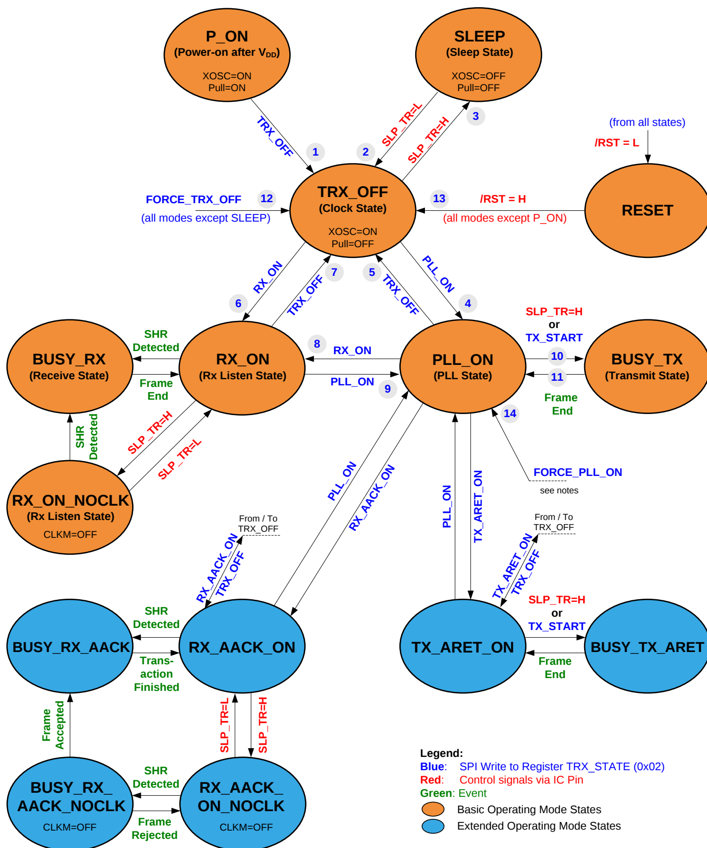
Figure 7-10. Extended Operating Mode State Diagram.
