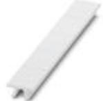
Zack marker strip, Strip, white, unlabeled, can be labeled with: PLOTMARK, CMS-P1-PLOTTER, mounting type: snap into tall marker groove, for terminal block width: 15.2 mm, lettering field size: 10.5 x 15.1 mm
