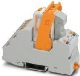
Pre-assembled relay module with push-in connection, consisting of: relay base, power contact relay, plug-in display/suppressor module, and retaining bracket. Contact type: 4 PDTs. Input voltage: 24 V AC
