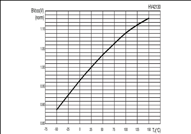
Figure 6. Normalized B_{V_{DS}} vs temperature
