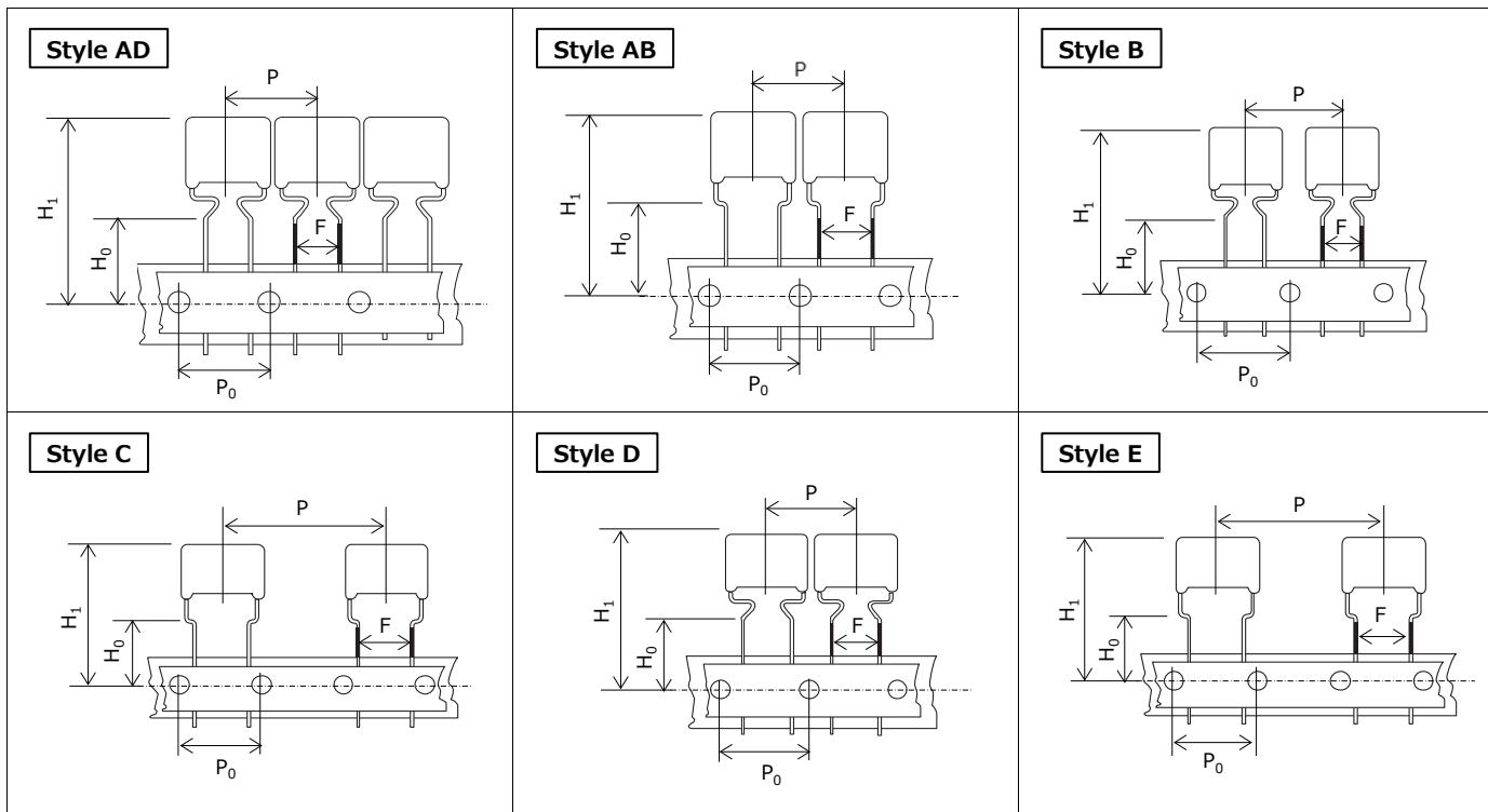
\*: H1 dimension is based on insertion machine "Panasert RH series" made by Panasonic.
