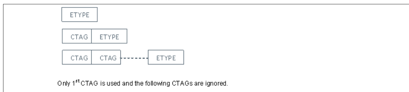
Figure 30 Supported Frame Formats when STAG is disabled
