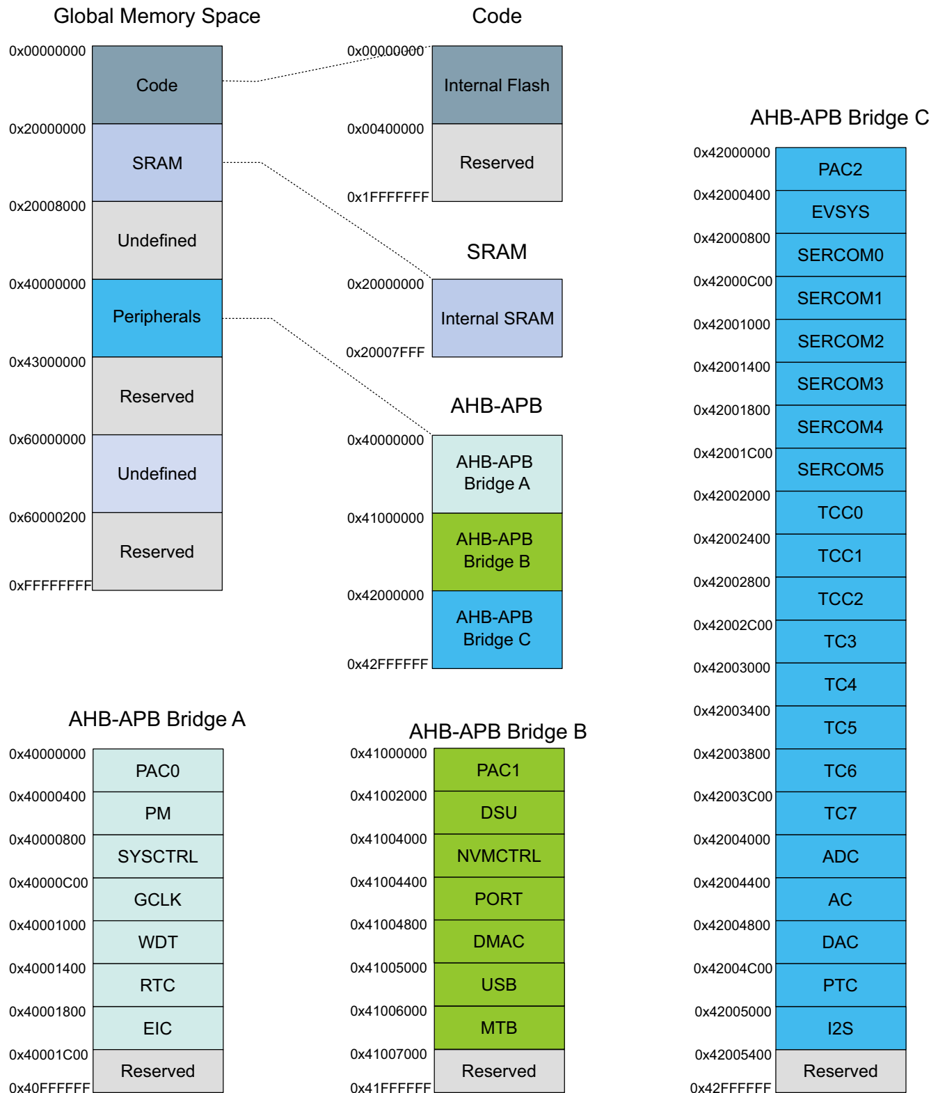
Figure 7-1. Atmel SAM D21 Product Mapping
